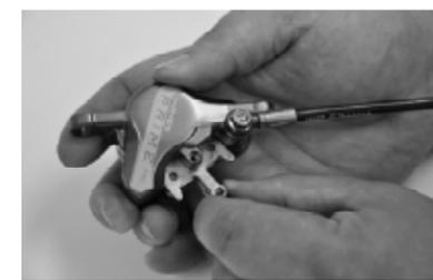
Figure 8. Retrait pads et "sandwich" ressort.
