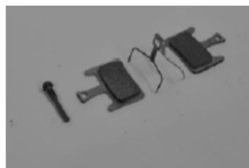
Figure 9. Brake pads, sandwich spring and pad retaining pin.
