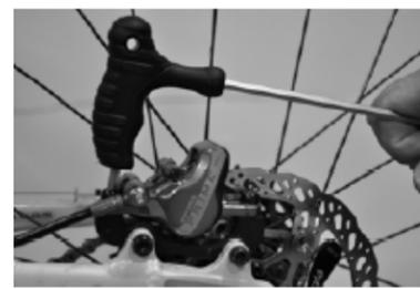
Figure 6. Mounting the caliper to the frame.
