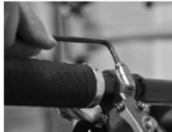
Figure 1. Tighten the side of the clamp with the Prime logo until there is no gap.
