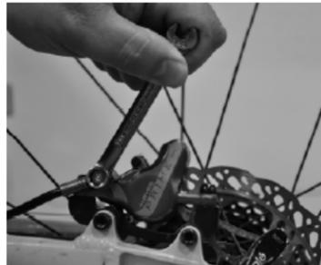
Figure 3. Loosen the banjo bolt to adjust the hose angle.
