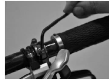
Figure 2. Torque the lower handlebar clamp screw to 30±5 in-lbs (3.37±0.55Nm)
