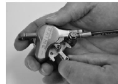
Figure 8. Removing pads and sandwich spring.
